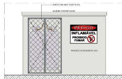
FACHADA 03 - CENTRAL GLP
