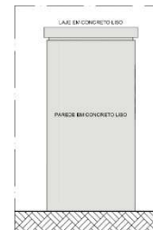
FACHADA 02 - CENTRAL GLP INDIVIDUAL
