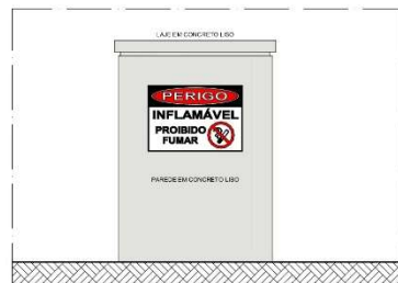
FACHADA 03 - CENTRAL GLP INDIVIDUAL
