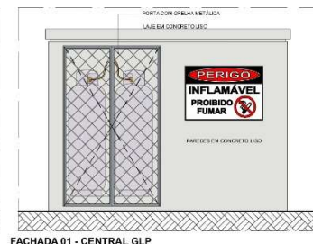
FACHADA 01 - CENTRAL GLP
